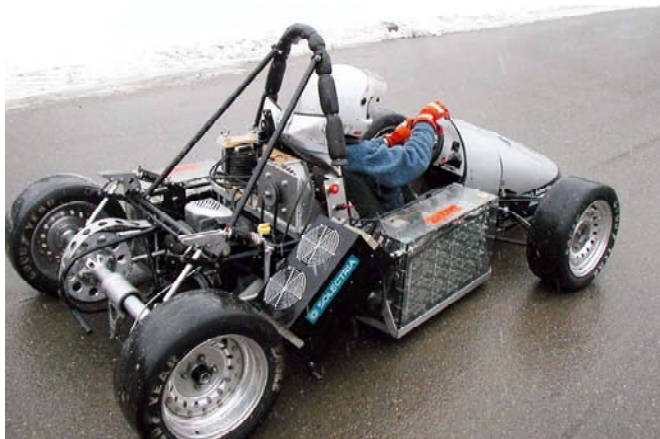
Figure 1. Completed vehicle. One of two ultracapacitor banks is visible to the driver's right.
