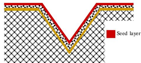
Fig. 5. A thin conductive metal seed layer that will be used for electroplating is deposited over the full wafer surface.
