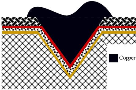
Fig. 7. Copper is electroplated into the V-grooves with the help of the seed layer.
