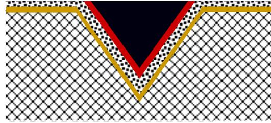
Fig. 8. A planarized wafer surface is achieved by chemical mechanical polishing to remove excess copper from electroplating.
