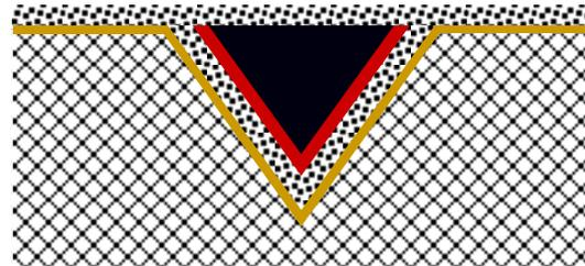
Fig. 9. More magnetic material is deposited to complete the V-groove inductor.
