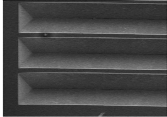
Fig. 3. SEM image showing the etched V-grooves in a silicon substrate.
