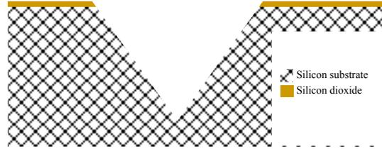
Fig. 2. Cross section showing the etched V-groove in a silicon substrate.
