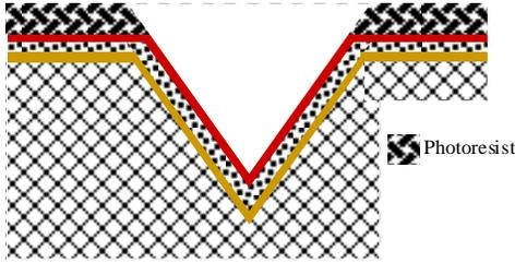
Fig. 6. Photoresist is spun and developed to expose the seed layer in the V-grooves.
