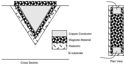
Fig. 1. Schematic diagram of V-groove inductor. Contact pads are indicated on the plan view by “bond wires”, but in practice the interconnection would be accomplished with another metal layer or solder bumps, to avoid high impedance and stray inductance associated with bond wires.
