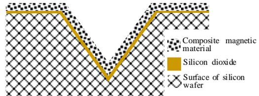
Fig. 4. Cross section showing the etched V-groove with two layers deposited on top of it: an insulating oxide layer followed by composite magnetic material.
