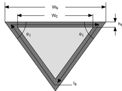
Fig. 4. Geometric parameters used in inductor calculations.  $h_s$  is the thickness of the magnetic material,  $W_s$  is the width of the magnetic material,  $W_c$  is the width of the copper conductor,  $l_s$  is the core flux path length, and  $\theta_1$  is the angle created during an anisotropic etch ( $54.7^\circ$ )
