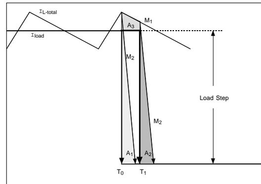
Fig. 2. Total inductor current and load current waveforms for a multi-phase converter with a load current step, assuming ideal switching control. Shaded area  $A_1$  represents excess charge transferred into the output capacitor if the load steps at time  $T_0$ . If the load steps at time  $T_1$ , the charge injected is area  $A_3$  plus  $A_2$ . Thus, the worst-case timing for the step is no longer coincident with the peak current.
